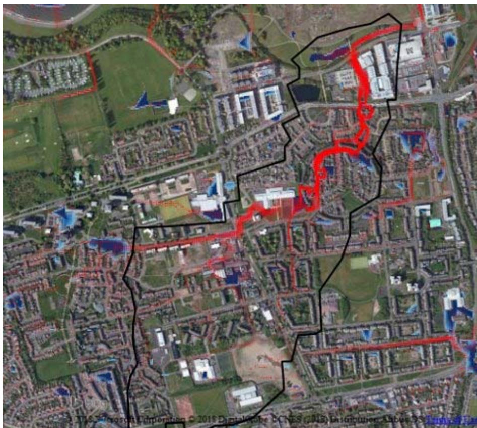
Figure 9. CityCat modelling of a 60 minute 100 years return period storm at Granton Pond catchment. Flow velocities are in red, water depths are in blue. The simulation snapshot is at the end of the event.
