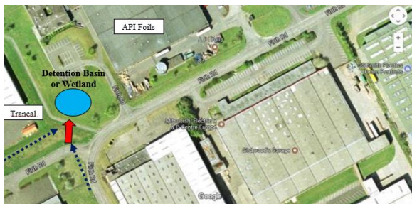
Figure 3: The proposed regional SUDS feature (Google DigitalGlobe 2018). Arrows show connecting swales.
